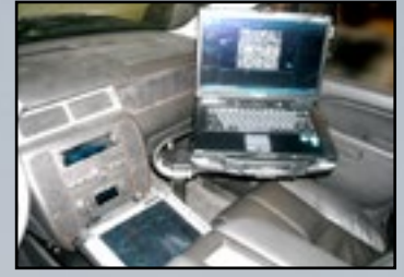
Wisdom C&C software on laptop (top) integrates with remote command center. CCU touchscreen computer (bottom) controls vehicle subsystems
