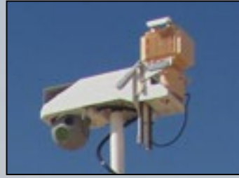
Sophisticated sensor array, consisting of a radar and a day/night PTZ camera is easily deployed in remote locations
